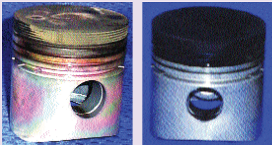
Figure 1 A SilcoKlean™1000-treated piston (left) shows dramatically less coke buildup than an untreated diesel piston (right). Data courtesy of The Pennsylvania State University.
